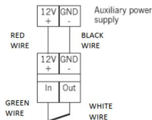
· Wiring diagram for the installation of more than one activator in series (maximum 4) and avoiding interference between them. To do so, the OUT synch. signal must be connected to the IN synch. signal of the following activator.
